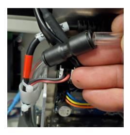
The AA tubing is held by a tubing coupler. To remove the tubing, press the tubing into the fixture. Then, while holding the retaining ring tight to the fixture, pull the AA tubing away from it.
