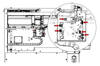
7. Connect the air assist tubing to the right side of the x-axis assembly:
