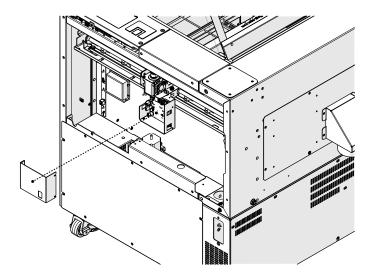
6. Disconnect the air assist tubing from the right side of the x-axis assembly:
