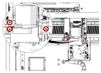
6. Connect the six (6) electrical harnesses on the drive board:
