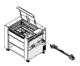
2. Place the x-axis assembly on the y-axis bearing blocks ensuring that it sits on the locator pins:
