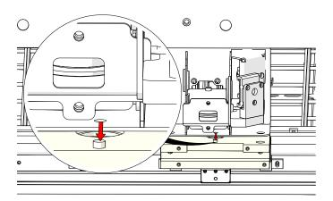
13. Slide the x-axis assembly out of the cabinet through the right side of the engraver:
