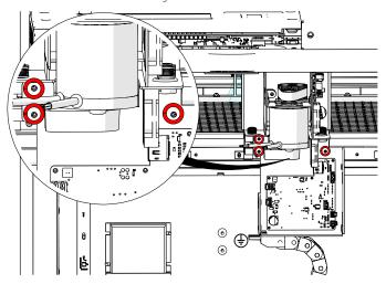
9. Remove the x-axis drive board and housing:
