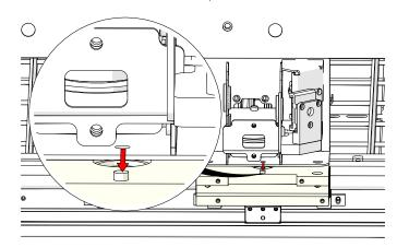
3. Install and tighten the four (4) fasteners that secure the x-axis assembly to the y-axis bearings. There are two (2) on the right side and two (2) on the left side:
