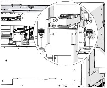
12. Gently lift on the x-axis assembly to free it from the locator pins on the y-axis bearing blocks:
