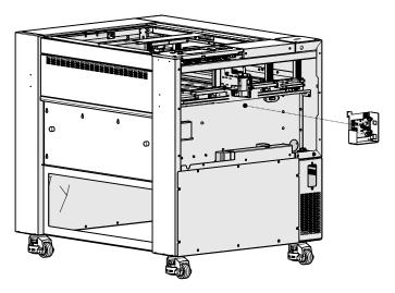
5. Install and tighten the three (3) Phillips screws that secure the x-axis drive board mounting bracket to the x-axis assembly:
