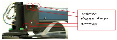
6. Detach the white ribbon cable. The white ribbon cable connects to the amplifier by a black connector. With the index finger, press the lever
