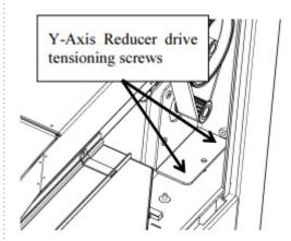
6. Once the reducer drive belt is loose, it can be removed from the machine.
