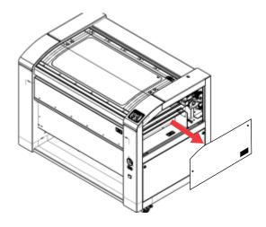
3. Remove the Exhaust Plenum assembly from the rear of the machine.
