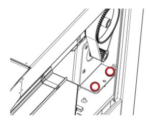
3. Apply sufficient tension to the Y-Axis belt so that the Y-Motor Bracket is roughly 1/2 inch from the bottom of the machine.
