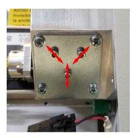
NOTE: Small adjustments can make a big difference in laser location. To avoid "loss" of the laser and red dot fire, use very small adjustments when attempting to center the burn mark. If at any point you are unable to get a burn mark or see the red dot diode, call Epilog Tech Support.
