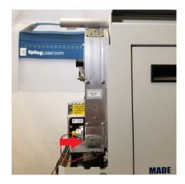
3. Adjustments of this mirror are made using the three (3) 3/32" allen head screws, each of which move the laser/red dot in a different direction on the target. The movement each screw controls are shown below:
